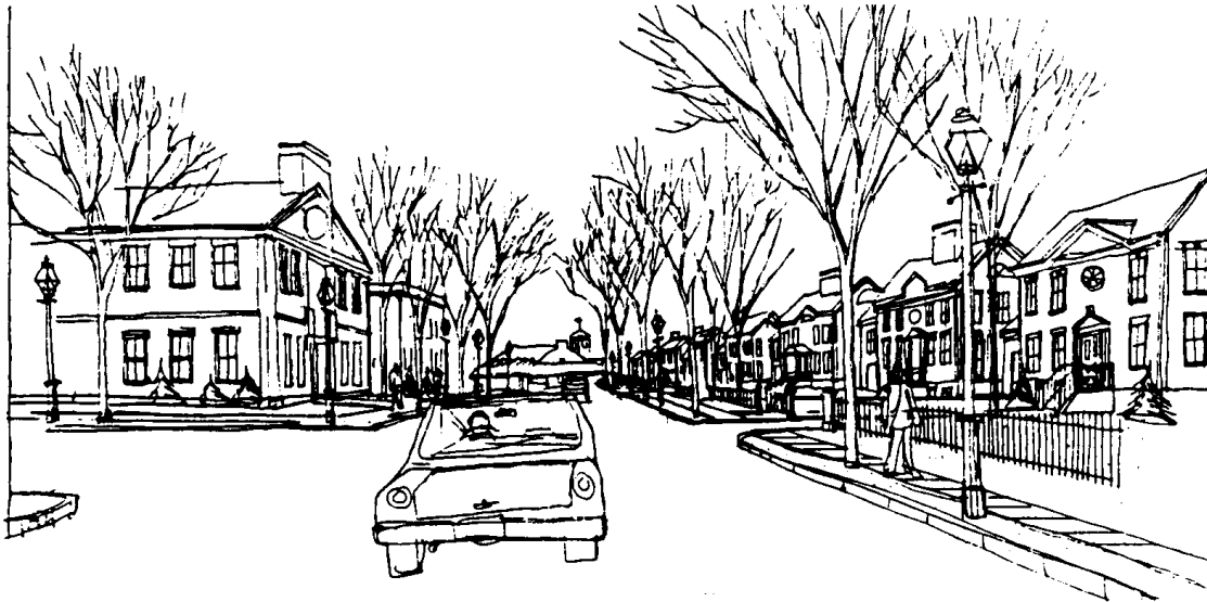
Illustration 59 — Buildings should define the streetscape through uniform setbacks along the build-to line.
