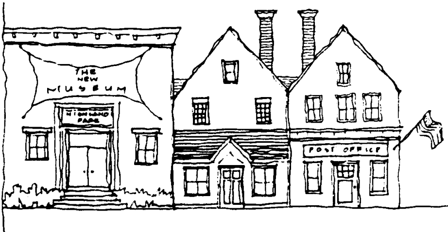
Illustration 74 — Gable roofs with a minimum nine twelfths (9/12) pitch should be used to the greatest extent possible. Other types of roofs should be appropriate to a building's architectural style.
