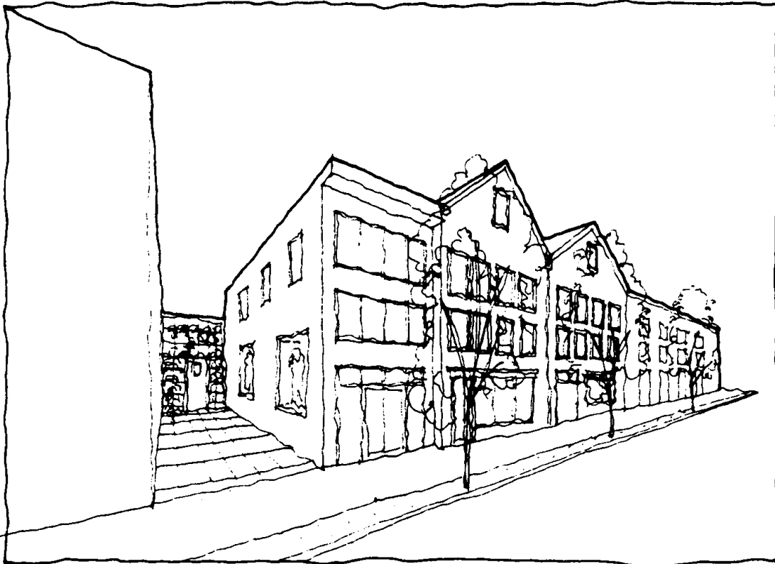
Illustration 76 — Blank, windowless walls should be articulated in order to reduce the negative effects of such walls.
