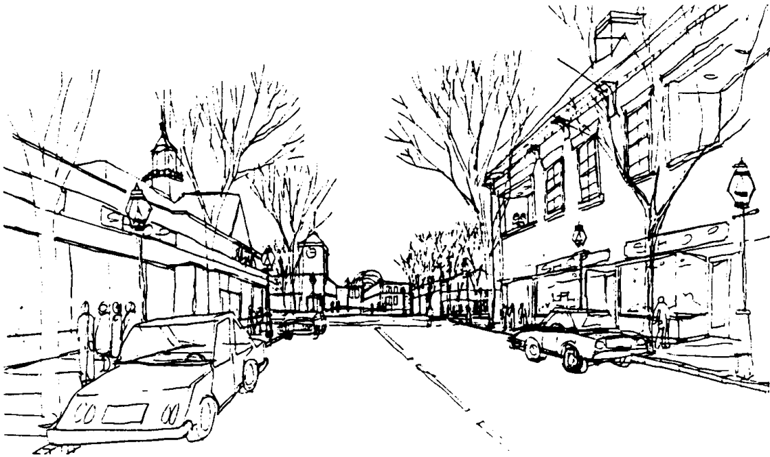
Illustration 79 — Storefronts should be integrally designed as part of the entire facade. Buildings with multiple storefronts should be architecturally compatible.
