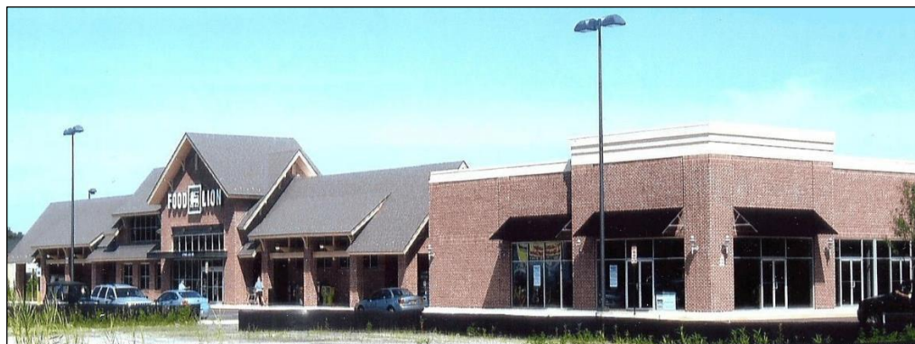
Sample of architectural articulation required of Destination Retail Use Buildings. The larger store on the left has architectural articulation as described. Compare this storefront with the smaller store on the right which is not articulated and appears proportionately larger.
