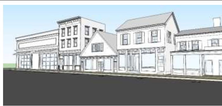
Typical commercial block building with simple massing, regular spacing of doors and windows, and a tall ground floor.
