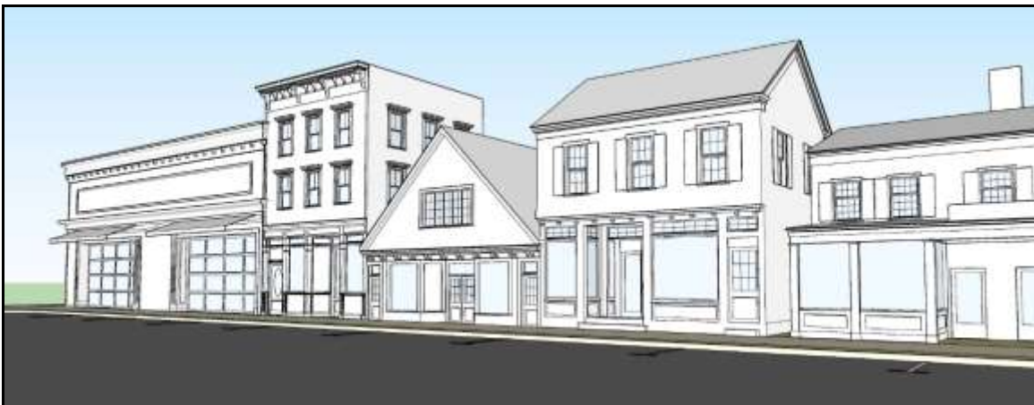
Large Building Massing. The public frontage of long buildings should be designed with a variety of minor, medium and major articulations and courtyard breaks to avoid the appearance of one long, uninterrupted facade.
